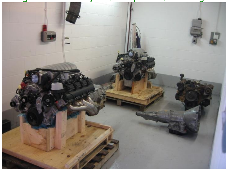
Brand new Chrysler V8 engines and automatic gearboxes ready to fit in place of the originals.
